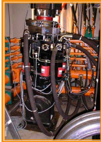
Figure 2. General view of a hydraulic actuator (MTS)
