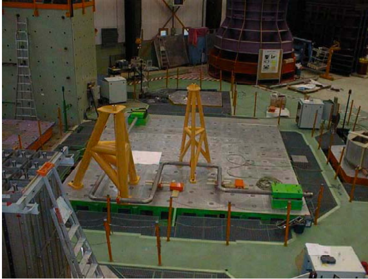
Figure 9. Piping system test (CEA Saclay - Azalée)
