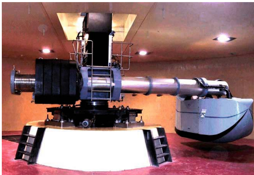
Figure 14. General view of a beam-type centrifuge (LCPC, Nantes France)
