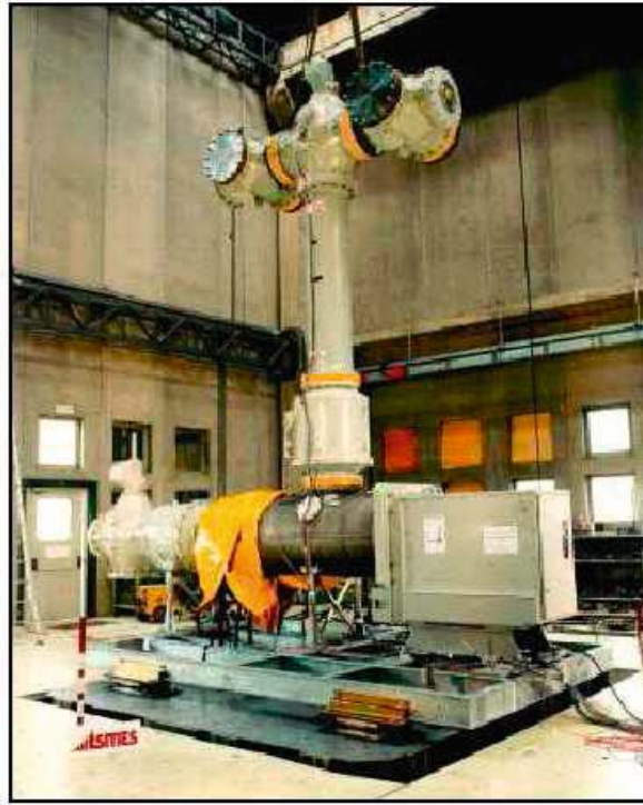
Figure 8. Qualification test of an isolator ( CESI-ISMES- Italy)
